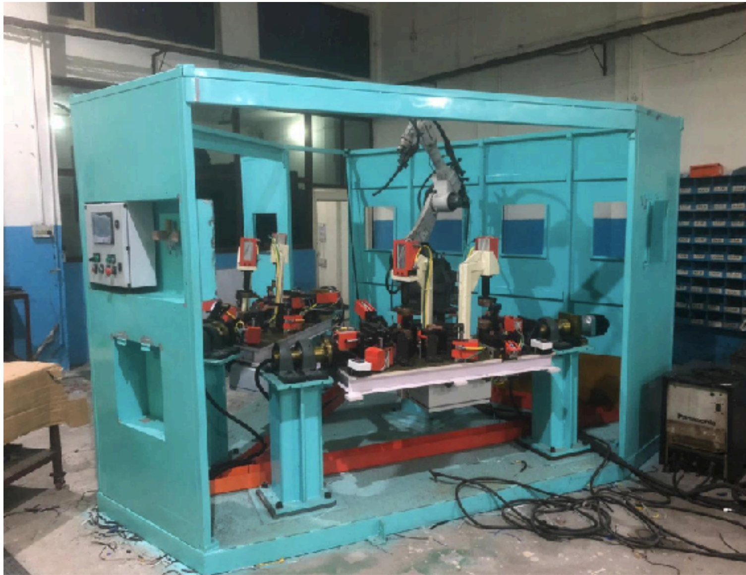
MIG WELDING ROBOTIC CELL FOR INDO AUTOTECH
